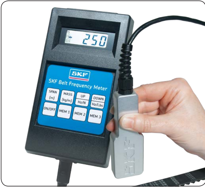
SKF Belt Frequency Meter PHL FM 10/400
